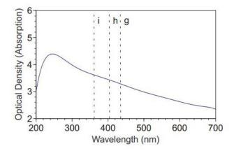
Optical Density 5 = 0.001% transmission Optical Density 4 = 0.01% transmission Optical Density 3 = 0.1% transmission
