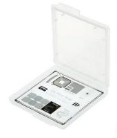
A photomask is an opaque plate or film with transparent areas that allow light to shine through in a defined pattern. They are commonly used in photolithography processes, but are also used in many other applications by a wide range of industries and technologies. They are made on Soda Lime glass, on Fused Silica (Quartz) and even on polyester film. The mask acts as a template, and is designed to optically transfer patterns to wafers or other substrates in order to fabricate devices of all types
