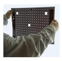
A photomask is an opaque plate or film with transparent areas that allow light to shine through in a defined pattern. They are commonly used in photolithography processes, but are also used in many other applications by a wide range of industries and technologies. They are made on Soda Lime glass, on Fused Silica (Quartz) and even on polyester film. The mask acts as a template, and is designed to optically transfer patterns to wafers or other substrates in order to fabricate devices of all types
