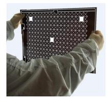
A photomask is an opaque plate or film with transparent areas that allow light to shine through in a defined pattern. They are commonly used in photolithography processes, but are also used in many other applications by a wide range of industries and technologies. They are made on Soda Lime glass, on Fused Silica (Quartz) and even on polyester film. The mask acts as a template, and is designed to optically transfer patterns to wafers or other substrates in order to fabricate devices of all types
