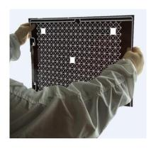
A Laser Photoplot is an opaque film with transparent areas that allow light to shine through in a defined pattern. They are commonly used in photolithography processes but are also used in many other applications by a wide range of industries and technologies. They are made on emulsion coated polyester film. The film acts as a template, and is designed to optically transfer patterns to other substrates in order to fabricate devices of all types
