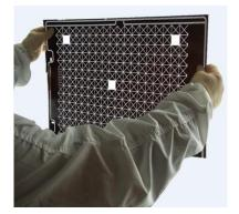
A Laser Photoplot is an opaque film with transparent areas that allow light to shine through in a defined pattern. They are commonly used in photolithography processes but are also used in many other applications by a wide range of industries and technologies. They are made on emulsion coated polyester film. The film acts as a template, and is designed to optically transfer patterns to other substrates in order to fabricate devices of all types
